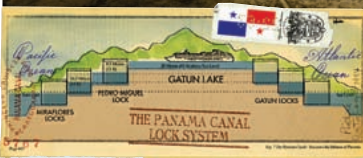
Top: Building of the Panama Canal Bottom: Panama Canal cross section
